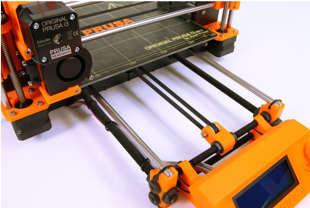
Pict. 32 - A properly tightened Y-axis belt under the heatbed
