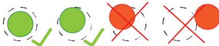
Pic. 7 - The probe must be inside the circles to successfully calibrate.
