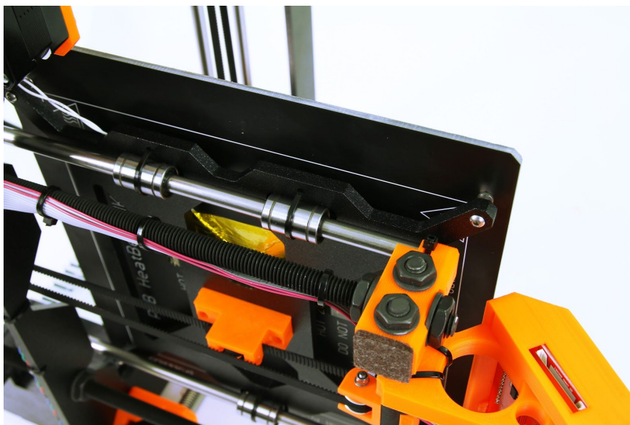
Pict. 35 - Properly tightened zipties under the heatbed
