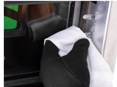
Image 62. Correct removal of the old and installing the new INFRARED HEATERS.
