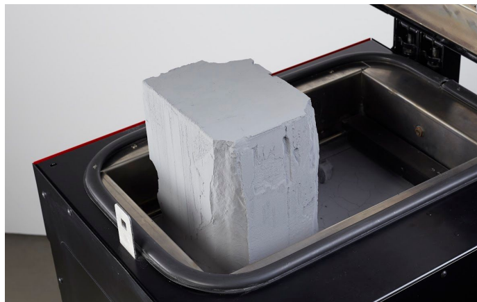
Image 38. A correct condition of the powder after printing (visible cracks on the surfaces of both BEDs).
