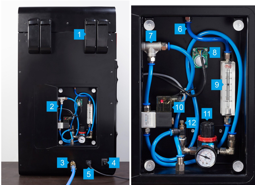
Image 3. View of the printer's gas installation.
