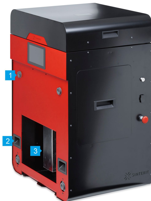
Image 4. View of the printer without front panel.
