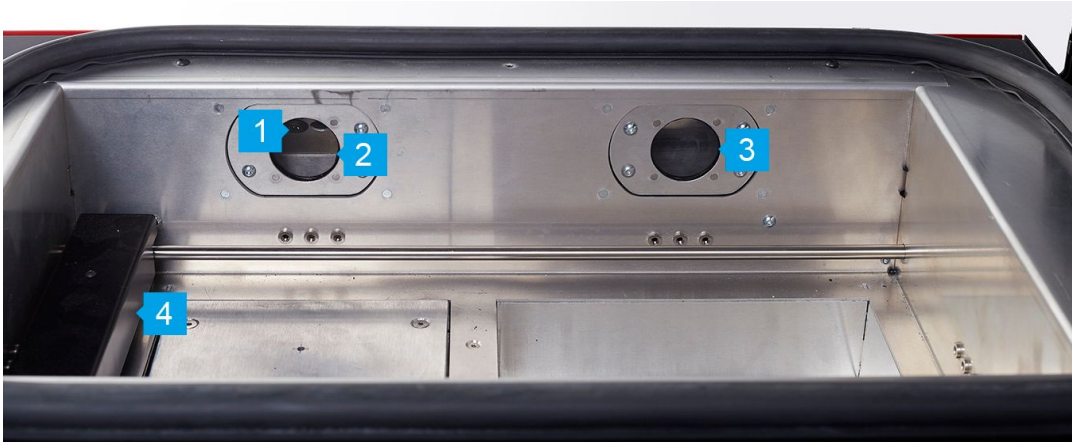
Image 7. Back view of the printer's inner chamber. 1.Embedded camera (captures image from the Print Bed) / 2.Print Bed pyrometer / 3.Feed Bed Pyrometer / 4.Recoater
