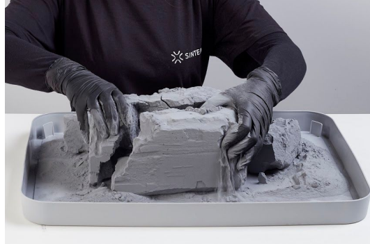
Images 39. A correct way of taking out the prints from the PRINT BED.
