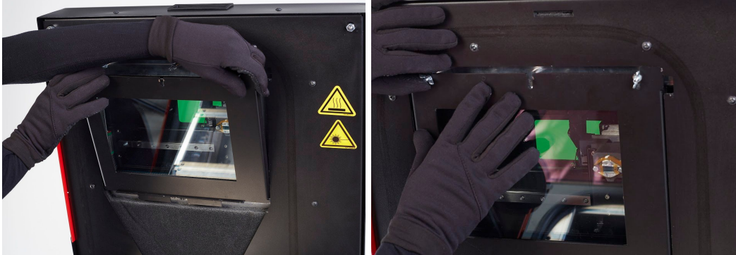
Image 58. Correct placement of the LASER PROTECTIVE GLASS on the HEATER MODULE.
