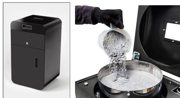
Image 54. Sieving the powder using Sinterit POWDER SIEVE.
