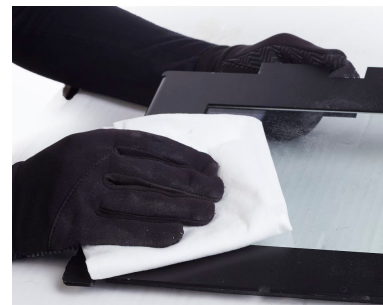
Image 15. Cleaning of LASER PROTECTIVE GLASS.
