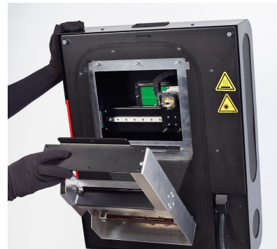
Image 13. Heater module - opening.
