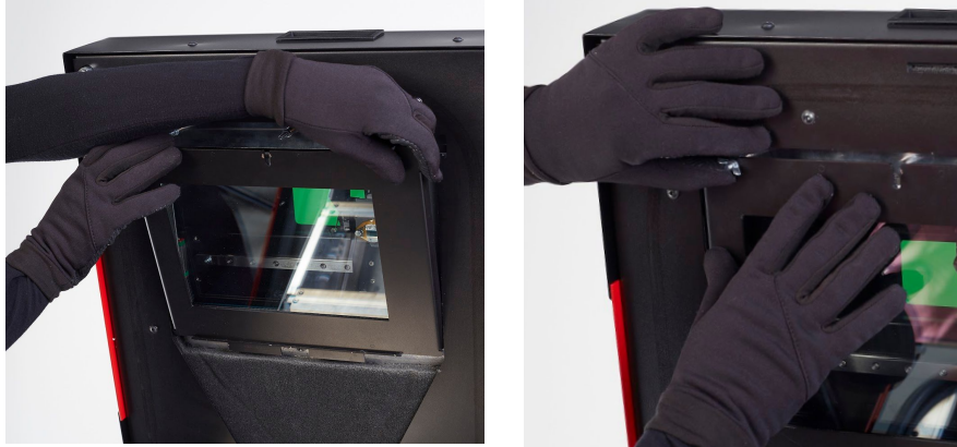
Image 16. Correct placement of the LASER PROTECTIVE GLASS on the heating module.
