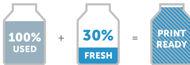
Image 56. The method of combining PA12 with refreshing ratio 30% after the printing.
