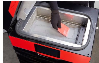
Image 27. Step 3. Equal distribution of powder on both BEDs
