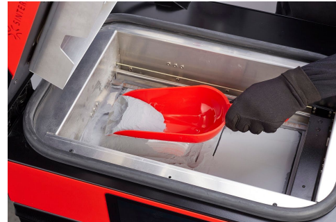
Image 45. Removing the powder from the FEED BED.
