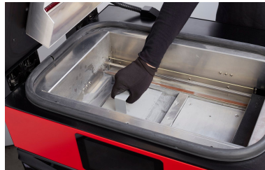
Image 26. Step 2. Compacting powder by gently pressing it.
