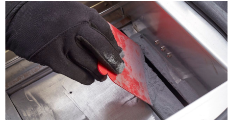
Image 48. Removing powder from PRINT BED to OVERFLOW BIN.
