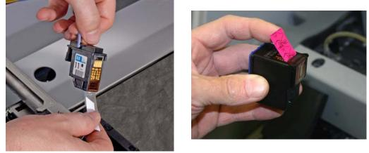
11. Insert the new printhead. Press down firmly on the top of the printhead, at the same side as the pogo pins, to securely fit the printhead into its slot.
