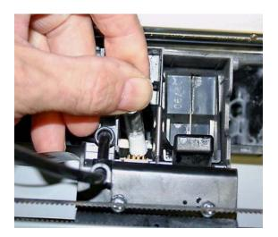
8. Wet a paper towel with distilled water and wipe the underside of the Carriage. Keep wiping until the towel picks up no more debris or ink.
