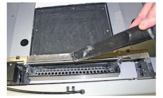
5. The vacuum will stop automatically if the Feeder becomes full, or you can push the Control Knob once to shut off the vacuum. If the Feeder does become full, the LCD displays:
