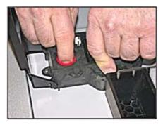
3. Remove the red cap. Add Cleaning Solution until the tank is HALF full. Do not overfill.
