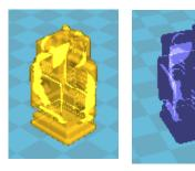
**Layers -** This view allows you to see the toolpath of the printhead so you can ensure that there are no skipped layers or gaps in the model. Drag the white button on the vertical layer selection bar to move up and down through the toolpath layers.
