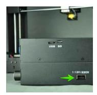
18. Ensure that the power switch is in the OFF position (O side depressed). Plug the C13 end of the included AC Power Cable into the C14 panel connector on the Power Supply/Control Box, then plug the other end into a nearby AC power outlet. Depress the I side of the power switch to power the printer ON.
