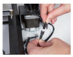
14. Insert the white connector on the shortest of the three cables into the corresponding white connector on the left side Z-axis stepper motor.
