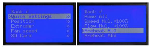
24. Monitor the temperatures of the extruder and plate on the LCD display. When they reach to within a few degrees of the targets, you are ready to insert filament. (Note that the display will still show *Preheat PLA*, even after the temperatures have reached the target values.) Carefully insert the included filament sample into the hole on the extruder, as shown.
